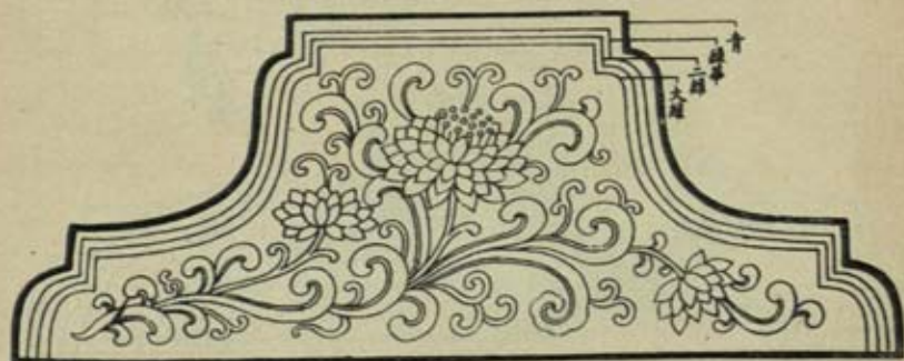
FIG. 2.—Versions of the same designs as those shown in Fig. 1, thus interpreted in the 1925 edition of Ying tsao fa shih . This edition includes counterparts printed in colour. It represents the border of the upper design in four hands, from without inwards: leaf green, pale pink, deeper pink and scarlet. The floral part of the upper design is in light and dark blues and greens. The border of the lower design is coloured from without inwards: dark blue, pale, middle and dark leaf green; while the floral part exhibits all three shades of blue, red and green.
